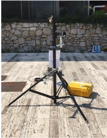
Figure 11. Portable microclimatic station for short-term outdoor monitoring located in an open space close to one of the two villas.
