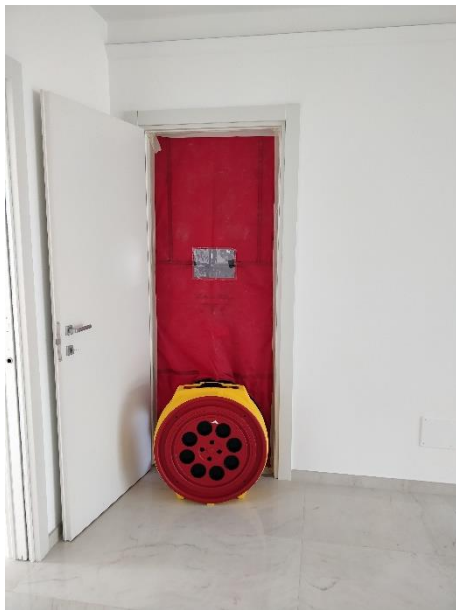
Figure 7. The Blower-Door test for the air permeability – infiltration - evaluation.
