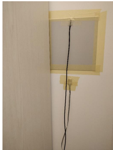
Figure 8. The U-value test for the thermal transmittance and heat flow evaluation.
