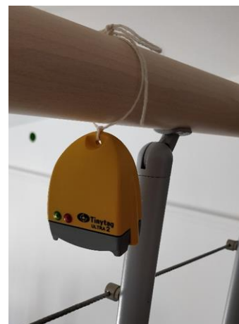
Figure 10. Tinytag probe for indoor air temperature monitoring used during the co-heating test.
