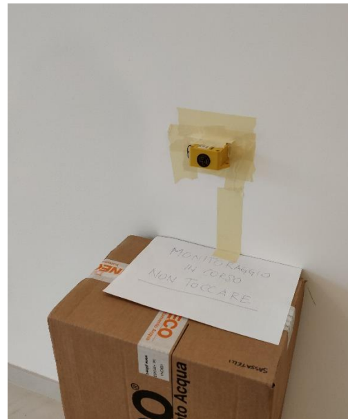
Figure 14. Tinytag probe for indoor air temperature and relative humidity measures used for the short-term monitoring.
