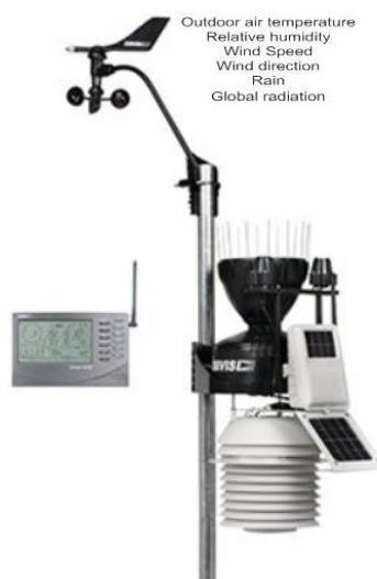
Figure 19. Weather station for climatic data collection by DAVIS.
