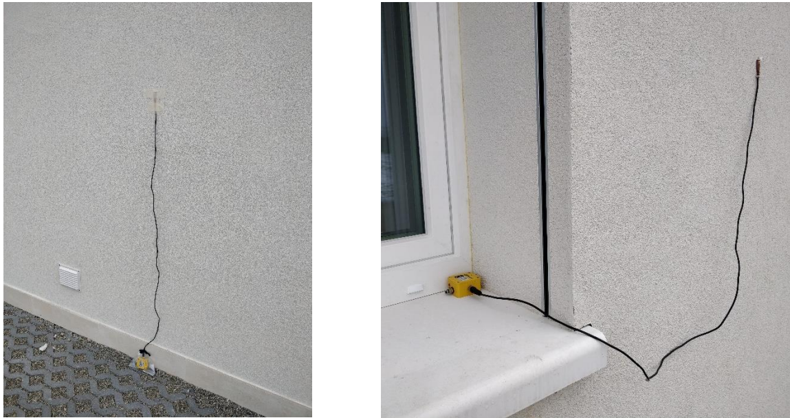
Figure 15. Short-term monitoring of the external walls surface temperature performed with Tinytag probes.
